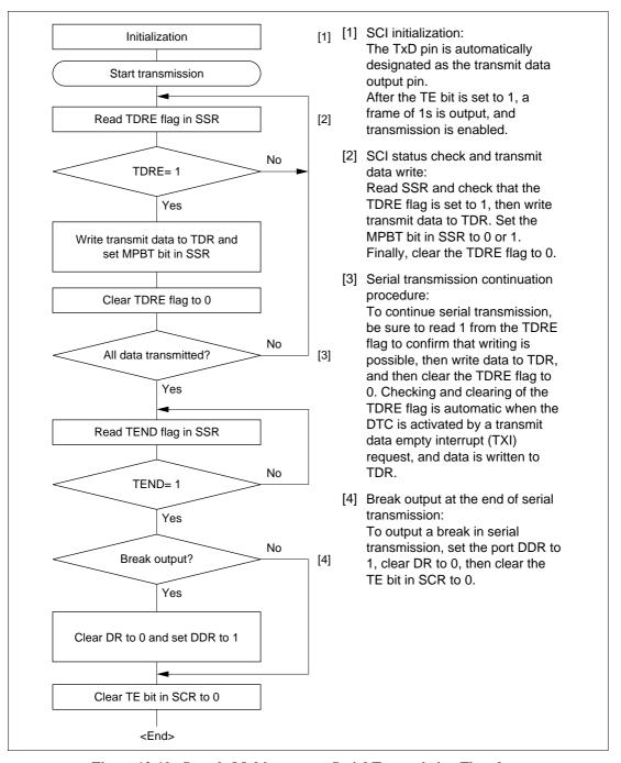
Figure 12-10 Sample Multiprocessor Serial Transmission Flowchart
