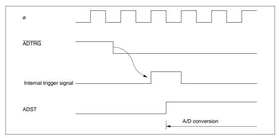
Figure 14-6 External Trigger Input Timing
