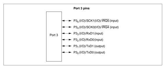
Figure 8-3 Port 3 Pin Functions
