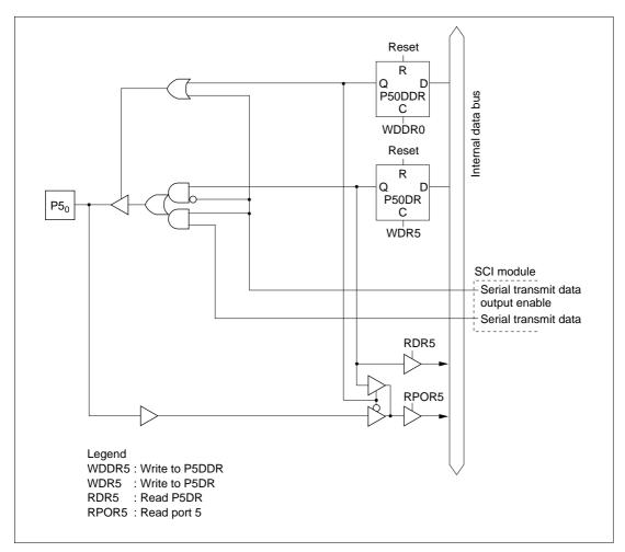
Figure C-5 (a) Port 5 Block Diagram (Pin P5<sub>0</sub>)
