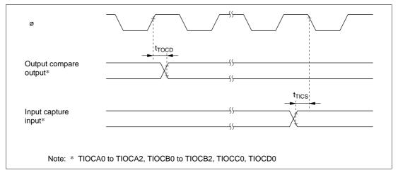
Figure 19-16 TPU Input/Output Timing
