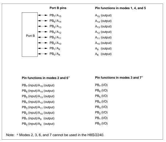
Figure 8-10 Port B Pin Functions
