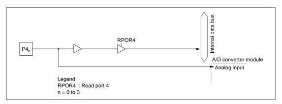
Figure C-4 Port 4 Block Diagram (Pins P4<sub>0</sub> to P4<sub>3</sub>)
