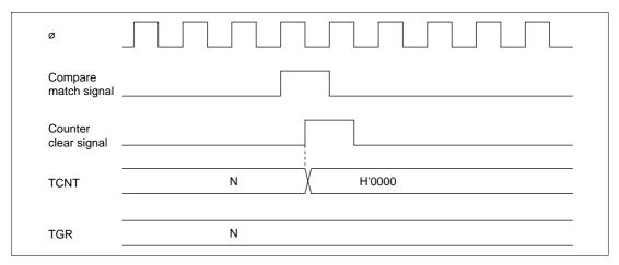
Figure 9-34 Counter Clear Timing (Compare Match)
