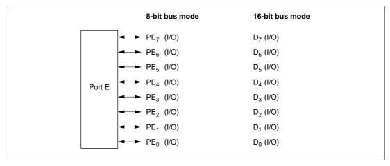
Figure 8-22 Port E Pin Functions (Modes 1, 2, 4, 5, and 6)
