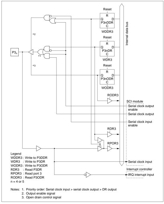
Figure C-3 (c) Port 3 Block Diagram (Pins P3<sub>4</sub> and P3<sub>5</sub>)
