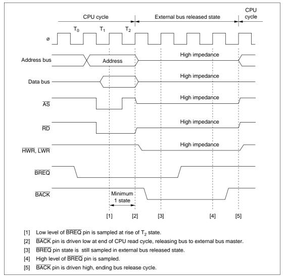
Figure 6-19 Bus-Released State Transition Timing
