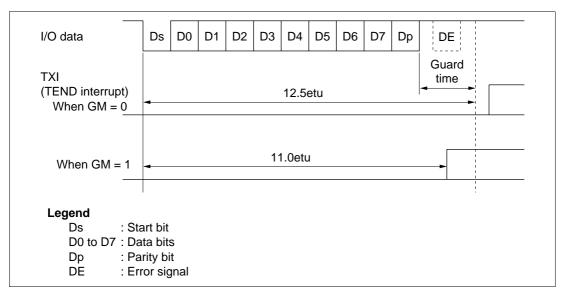
Figure 13-6 TEND Flag Generation Timing in Transmission Operation
