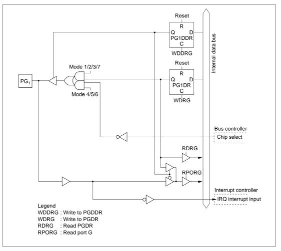
Figure C-12 (b) Port G Block Diagram (Pin PG<sub>1</sub>)
