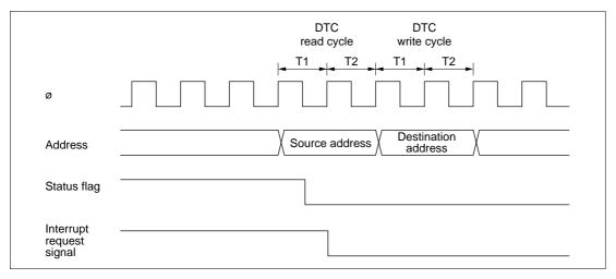
Figure 9-43 Timing for Status Flag Clearing by DTC Activation
