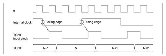
Figure 9-30 Count Timing in Internal Clock Operation
