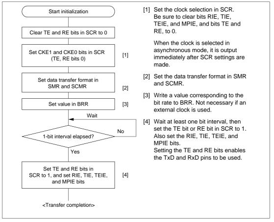
Figure 12-4 Sample SCI Initialization Flowchart
