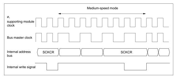
Figure 18-1 Medium-Speed Mode Transition and Clearance Timing
