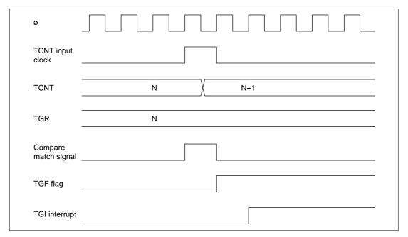
Figure 9-38 TGI Interrupt Timing (Compare Match)
