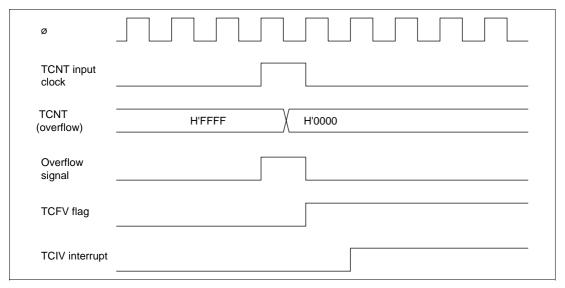
Figure 9-40 TCIV Interrupt Setting Timing
