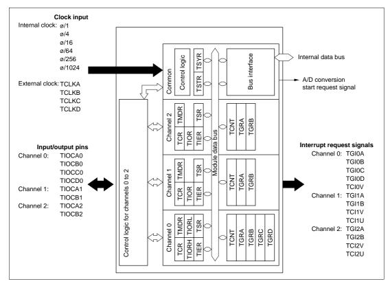
Figure 9-1 Block Diagram of TPU
