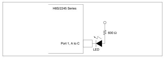
Figure 19-2 LED Drive Circuit (Example)
