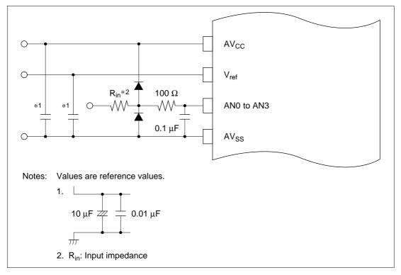
Figure 14-7 Example of Analog Input Protection Circuit
