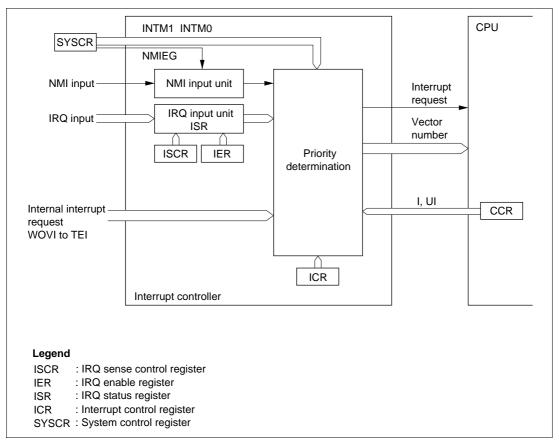
Figure 5-1 Block Diagram of Interrupt Controller
