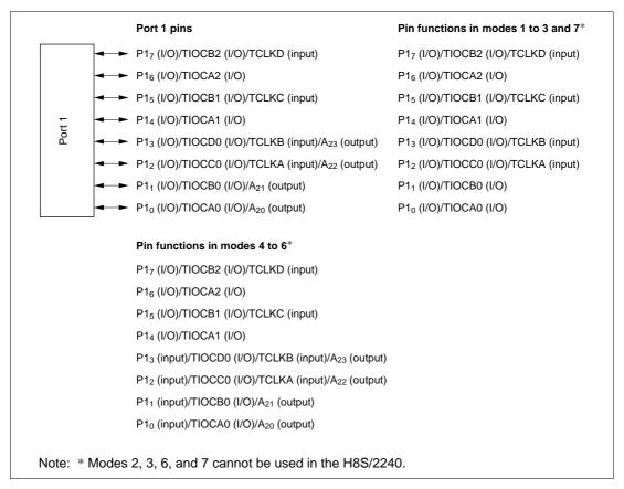
Figure 8-1 Port 1 Pin Functions
