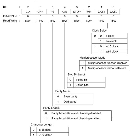
Note:  $^{*}$  When 7-bit data is selected, the MSB (bit 7) of TDR is not transmitted.
