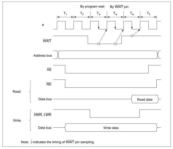
Figure 6-14 Example of Wait State Insertion Timing
