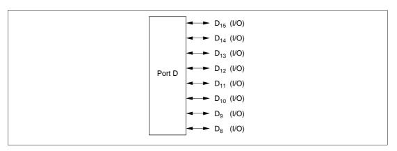
Figure 8-19 Port D Pin Functions (Modes 1, 2, 4, 5, and 6)
