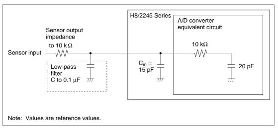
Figure 14-11 Example of Analog Input Circuit
