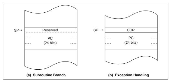
Figure 2-5 Stack Structure in Advanced Mode
