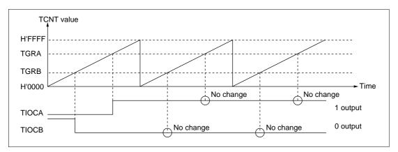
Figure 9-10 Example of 0 Output/1 Output Operation
