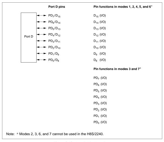
Figure 8-18 Port D Pin Functions
