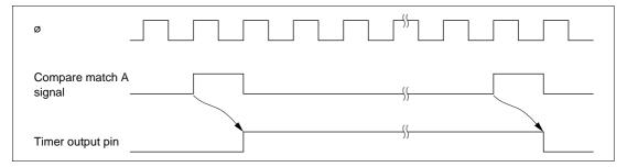
Figure 10-5 Timing of Timer Output
