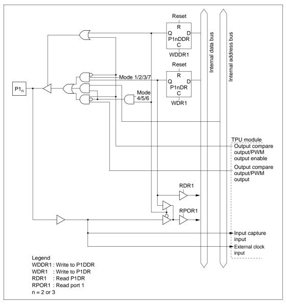
Figure C-1 (b) Port 1 Block Diagram (Pins P1<sub>2</sub> and P1<sub>3</sub>)
