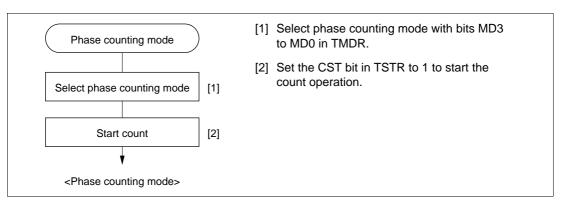
Figure 9-25 Example of Phase Counting Mode Setting Procedure
