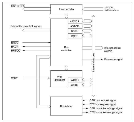
Figure 6-1 Block Diagram of Bus Controller
