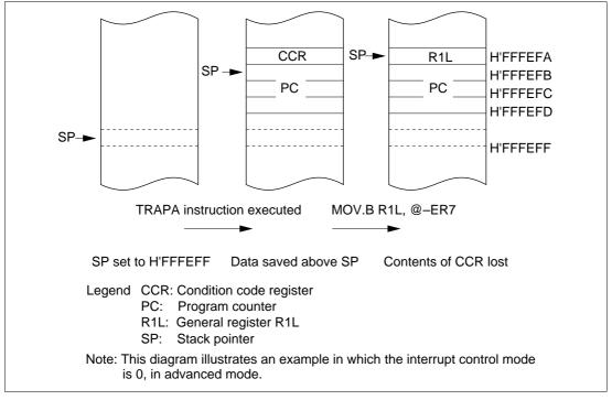
Figure 4-6 Operation when SP Value is Odd
