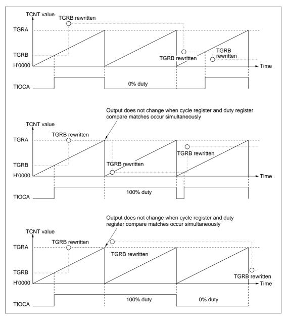
Figure 9-24 Example of PWM Mode Operation (3)
