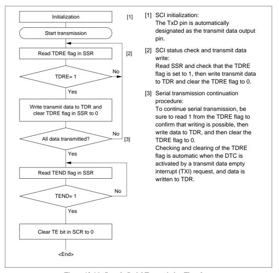
Figure 12-16 Sample Serial Transmission Flowchart
