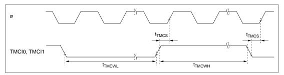
Figure 19-19 8-Bit Timer Clock Input Timing
