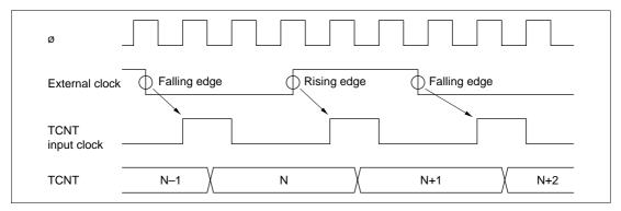
Figure 9-31 Count Timing in External Clock Operation
