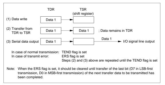
Figure 13-5 Relation Between Transmit Operation and Internal Registers
