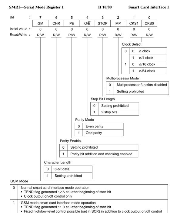
Note: etu (Elementary Time Unit): Interval for transfer of one bit
