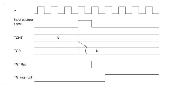
Figure 9-39 TGI Interrupt Timing (Input Capture)
