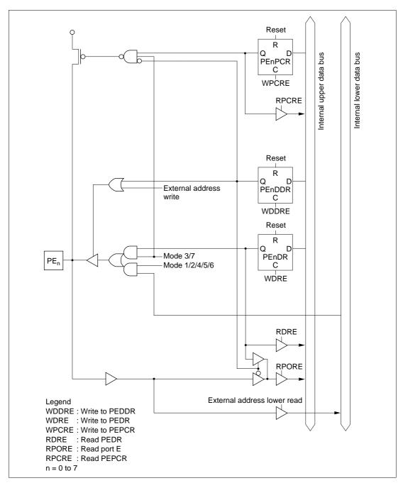
Figure C-10 Port E Block Diagram (Pin PE<sub>n</sub>)
