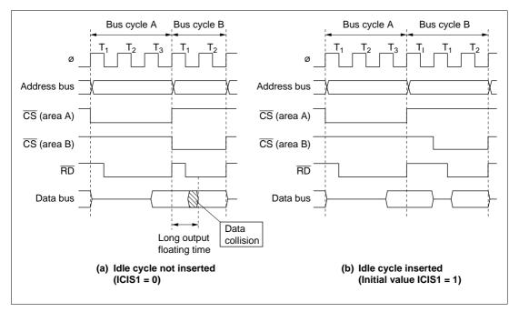
Figure 6-16 Example of Idle Cycle Operation (1)
