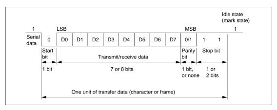
Figure 12-2 Data Format in Asynchronous Communication (Example with 8-Bit Data, Parity, Two Stop Bits)
