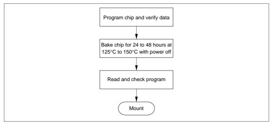
Figure 16-6 Recommended Screening Procedure
