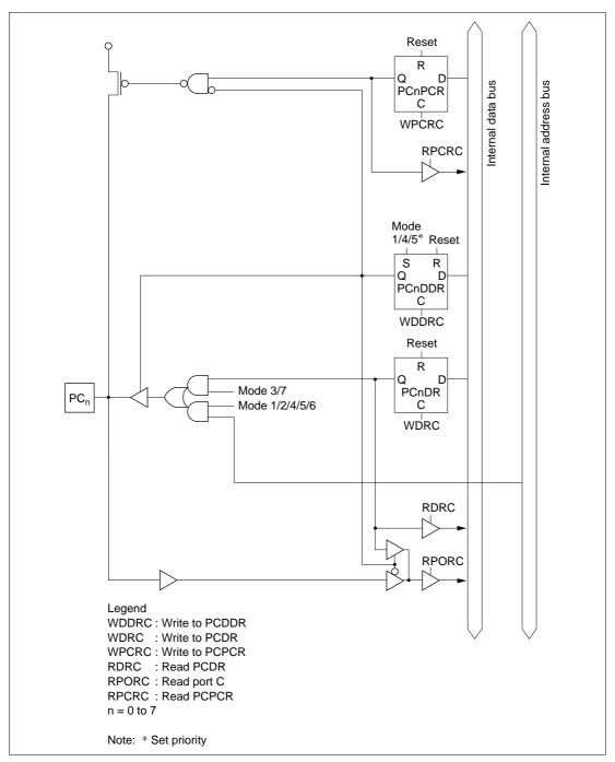
Figure C-8 Port C Block Diagram (Pin PC<sub>n</sub>)
