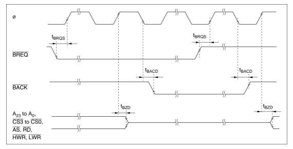
Figure 19-13 External Bus Release Timing
