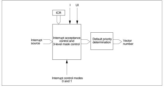
Figure 5-4 Block Diagram of Interrupt Control Operation
