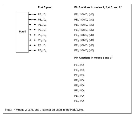
Figure 8-21 Port E Pin Functions
