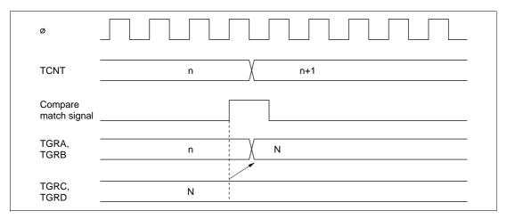
**Figure 9-36 Buffer Operation Timing (Compare Match)**
