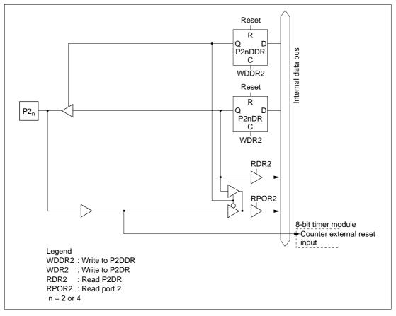
Figure C-2 (b) Port 2 Block Diagram (Pins P2<sub>2</sub> and P2<sub>4</sub>)
