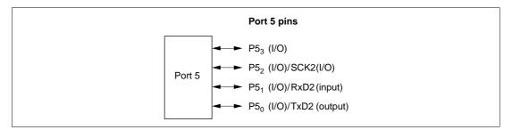
Figure 8-5 Port 5 Pin Functions
