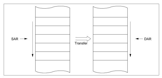
Figure 7-6 Memory Mapping in Normal Mode
