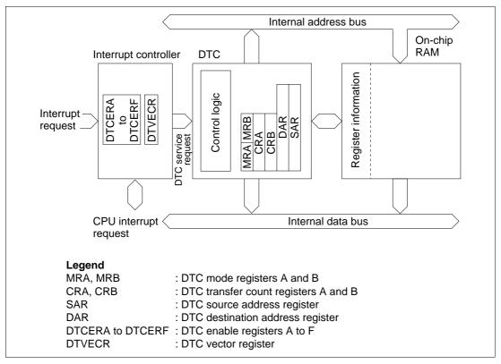
Figure 7-1 Block Diagram of DTC
