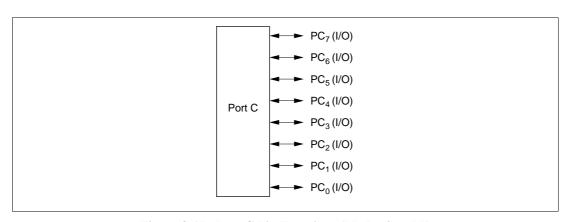
Figure 8-17 Port C Pin Functions (Modes 3 and 7)
