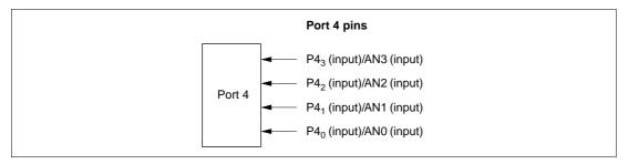
Figure 8-4 Port 4 Pin Functions
