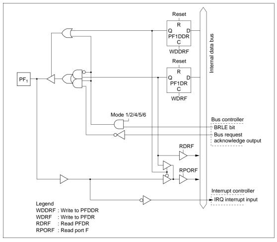
Figure C-11 (b) Port F Block Diagram (Pin PF<sub>1</sub>)
