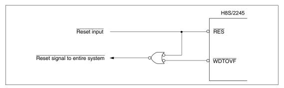
Figure 11-9 Circuit for System Reset by WDTOVF Signal (Example)
