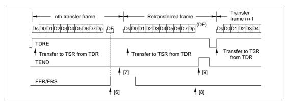
Figure 13-12 Retransfer Operation in SCI Transmit Mode
