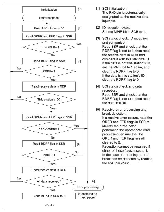
Figure 12-12 Sample Multiprocessor Serial Reception Flowchart
