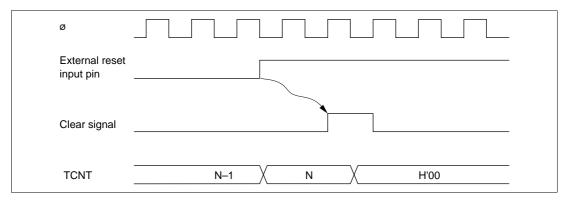
Figure 10-7 Timing of External Reset
