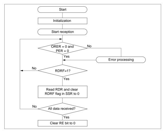
Figure 13-7 Example of Reception Processing Flow
