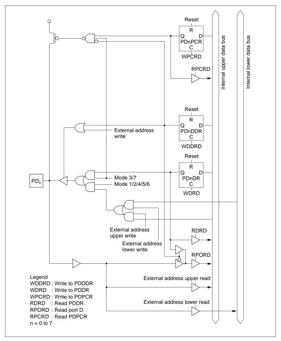
Figure C-9 Port D Block Diagram (Pin PD<sub>n</sub>)
