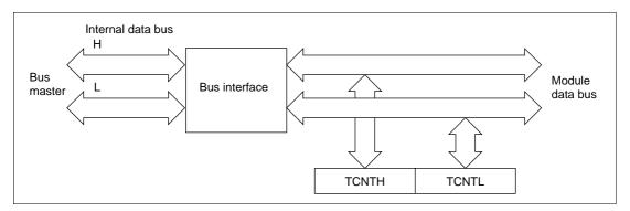
Figure 9-2 16-Bit Register Access Operation [Bus Master  $\leftrightarrow$  TCNT (16 Bits)]
