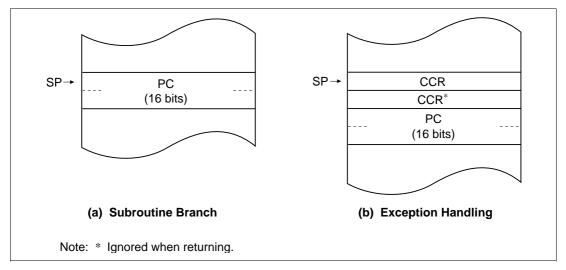
Figure 2-3 Stack Structure in Normal Mode
