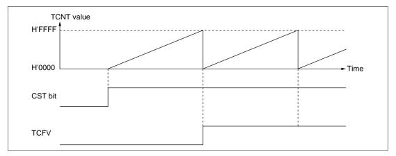
Figure 9-7 Free-Running Counter Operation
