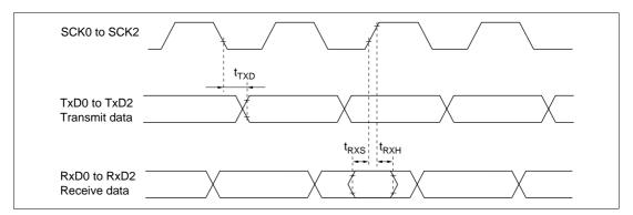
Figure 19-23 SCI Input/Output Timing Synchronous Mode
