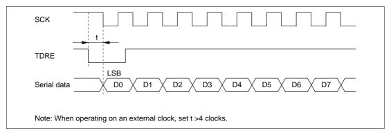
Figure 12-22 Example of Clocked Synchronous Transmission by DTC
