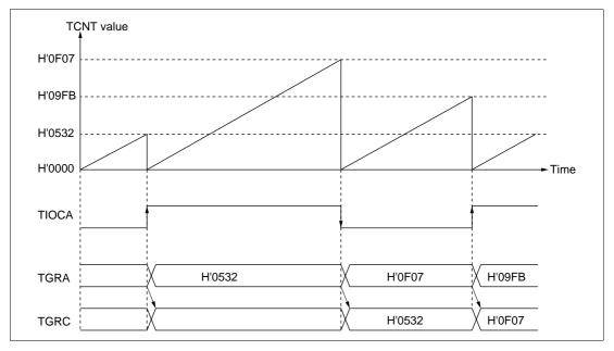
Figure 9-20 Example of Buffer Operation (2)
