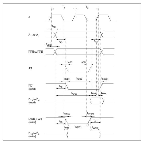
Figure 19-8 Basic Bus Timing (Two-State Access)
