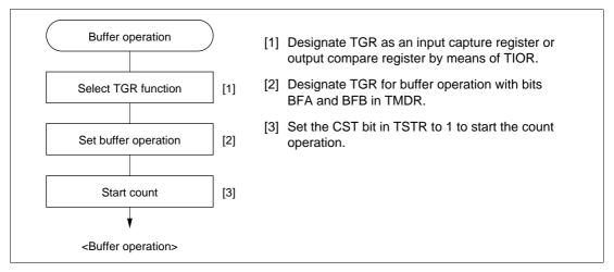
Figure 9-18 Example of Buffer Operation Setting Procedure
