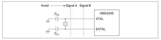
Figure 17-4 Example of Incorrect Board Design
