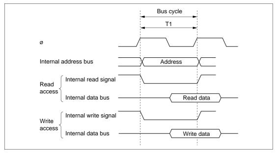
Figure 2-17 On-Chip Memory Access Cycle
