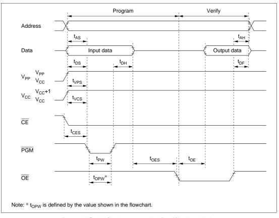
Figure 16-5 PROM Programming/Verification Timing
