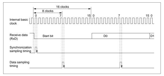
Figure 12-21 Receive Data Sampling Timing in Asynchronous Mode
