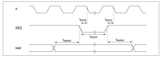
Figure 19-6 Reset Input Timing
