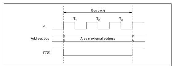
Figure 6-3 CSn Signal Output Timing (n = 0 to 3)
