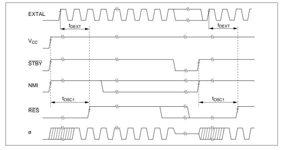
Figure 19-5 Oscillator Settling Timing
