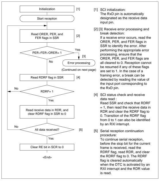
Figure 12-7 Sample Serial Reception Data Flowchart
