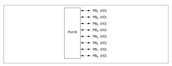
Figure 8-13 Port B Pin Functions (Modes 3 and 7)
