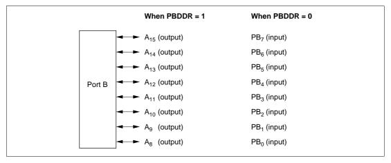
Figure 8-12 Port B Pin Functions (Modes 2 and 6)
