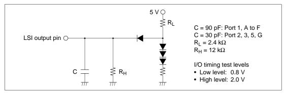
Figure 19-3 Output Load Circuit
