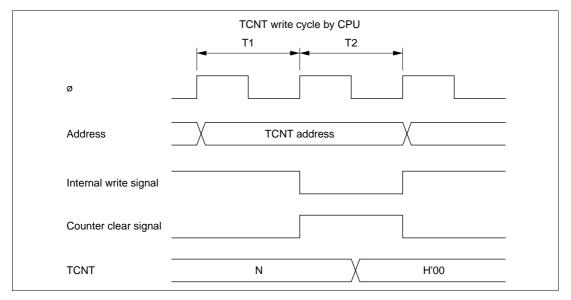
Figure 10-10 Contention between TCNT Write and Clear
