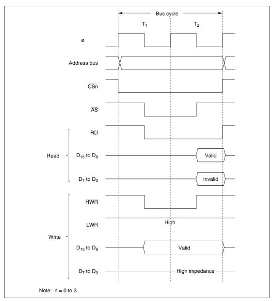
Figure 6-6 Bus Timing for 8-Bit 2-State Access Space
