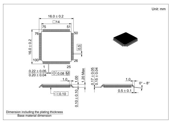
Figure H-2 TFP-100B Package Dimensions
