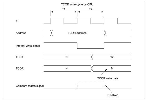
Figure 10-12 Contention between TCOR Write and Compare Match
