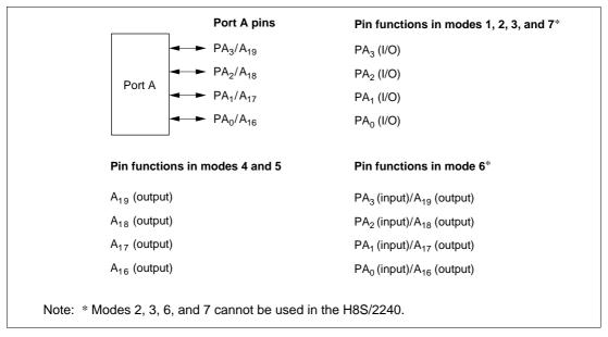
Figure 8-6 Port A Pin Functions
