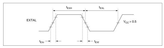
Figure 17-6 External Clock Input Timing
