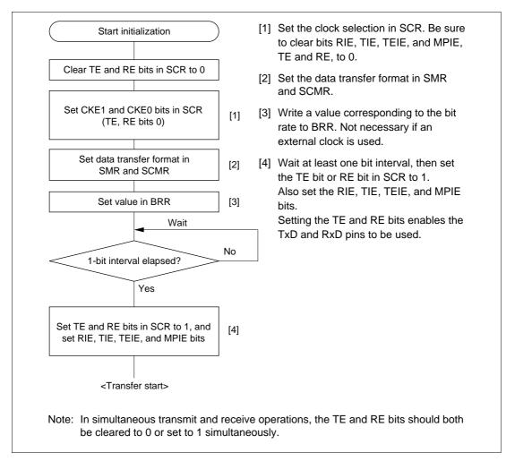
Figure 12-15 Sample SCI Initialization Flowchart
