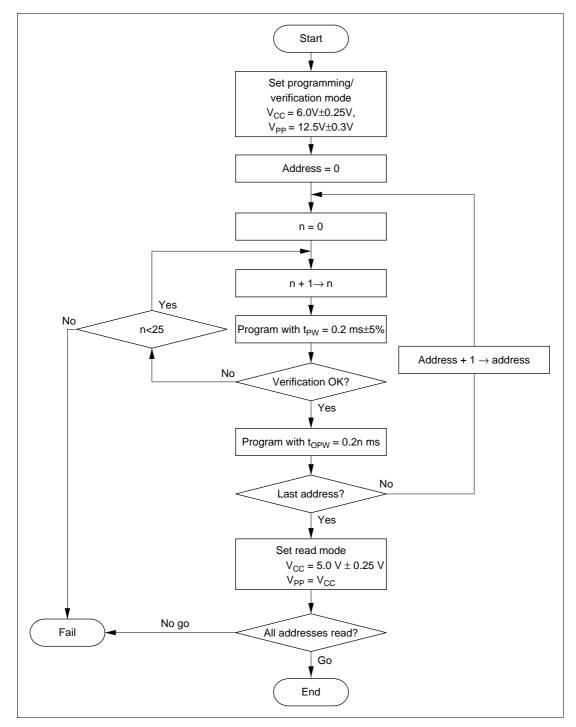
Figure 16-4 High-Speed Programming Flowchart
