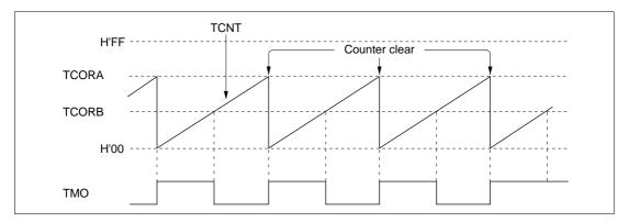
Figure 10-9 Example of Pulse Output
