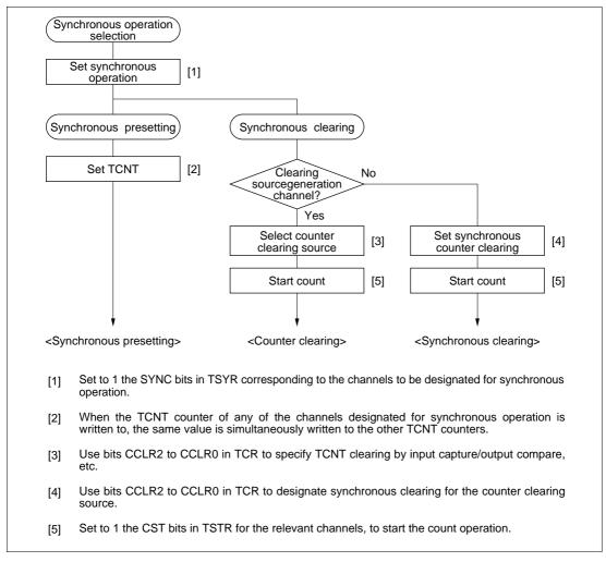
Figure 9-14 Example of Synchronous Operation Setting Procedure
