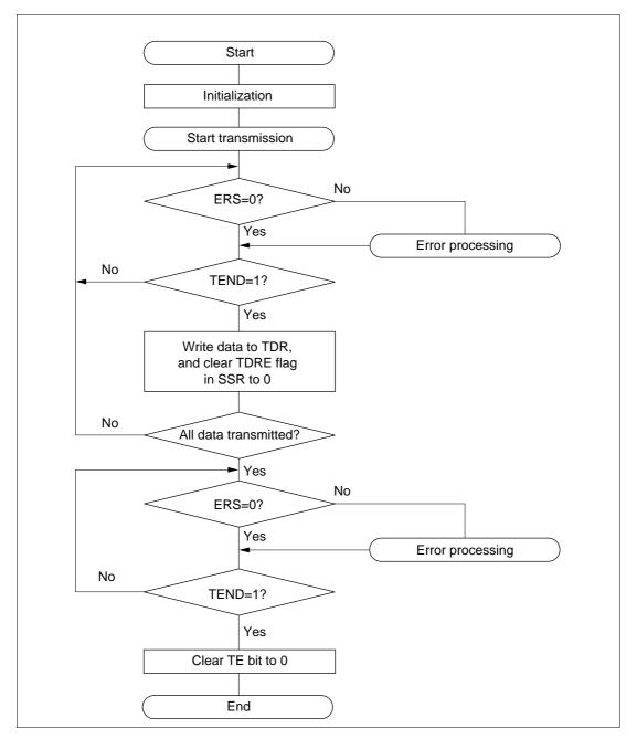
Figure 13-4 Example of Transmission Processing Flow
