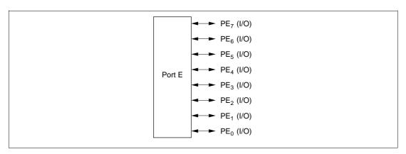
Figure 8-23 Port E Pin Functions (Modes 3 and 7)
