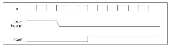
Figure 5-3 Timing of Setting IRQnF
