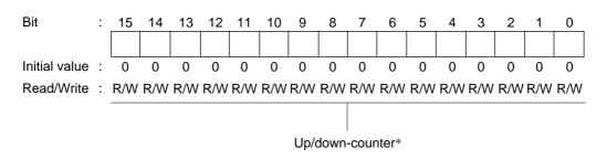
Note: \* This timer counter can be used as an up/down-counter only in phase counting mode or when performing overflow/underflow counting on another channel. In other cases it functions as an up-counter.
