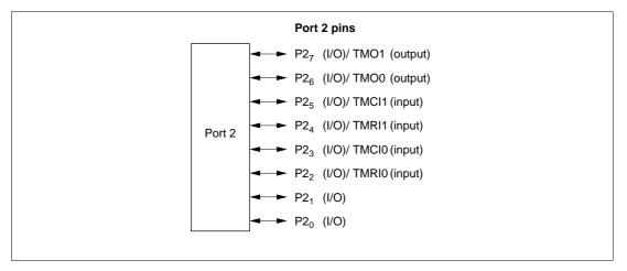
Figure 8-2 Port 2 Pin Functions
