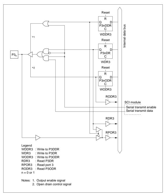
Figure C-3 (a) Port 3 Block Diagram (Pins P3<sub>0</sub> and P3<sub>1</sub>)
