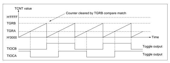
Figure 9-11 Example of Toggle Output Operation
