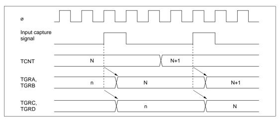
Figure 9-37 Buffer Operation Timing (Input Capture)
