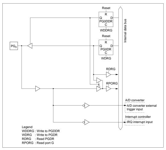
Figure C-12 (a) Port G Block Diagram (Pin PG<sub>0</sub>)
