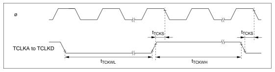
Figure 19-17 TPU Clock Input Timing
