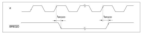
Figure 19-14 External Bus Request Output Timing
