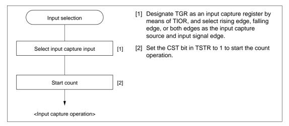
Figure 9-12 Example of Input Capture Operation Setting Procedure
