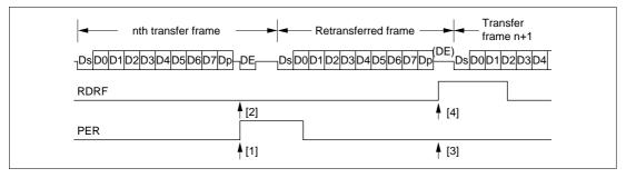
Figure 13-11 Retransfer Operation in SCI Receive Mode
