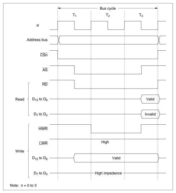
Figure 6-7 Bus Timing for 8-Bit 3-State Access Space
