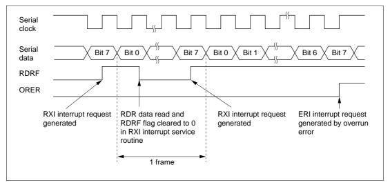
Figure 12-19 Example of SCI Operation in Reception
