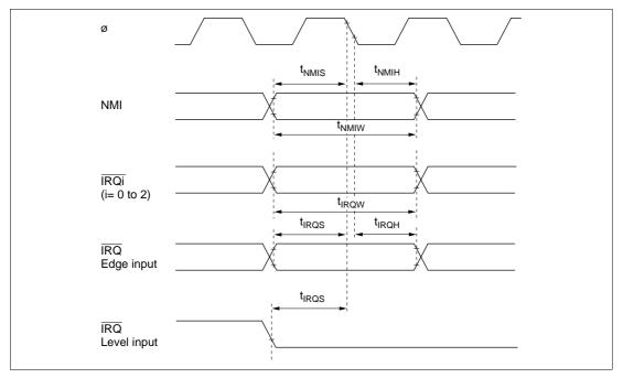
Figure 19-7 Interrupt Input Timing
