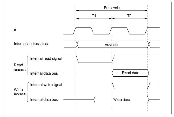
Figure 2-19 On-Chip Supporting Module Access Cycle
