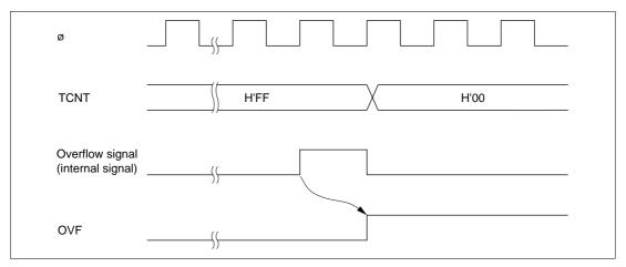
Figure 11-6 Timing of Setting of OVF
