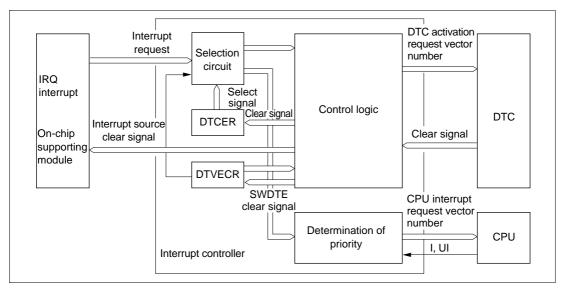
Figure 5-10 Interrupt Control for DTC
