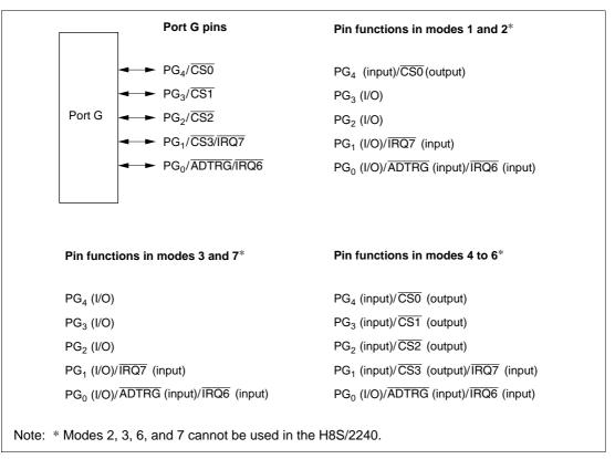
Figure 8-25 Port G Pin Functions
