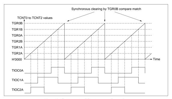
Figure 9-15 Example of Synchronous Operation
