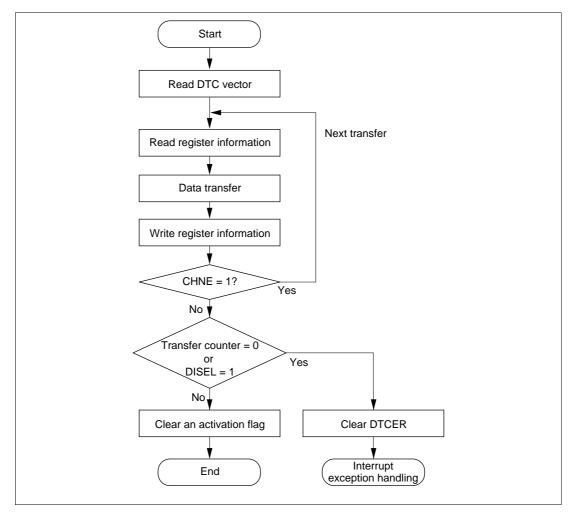
Figure 7-2 Flowchart of DTC Operation
