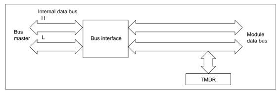
Figure 9-4 8-Bit Register Access Operation [Bus Master  $\leftrightarrow$  TMDR (Lower 8 Bits)]
