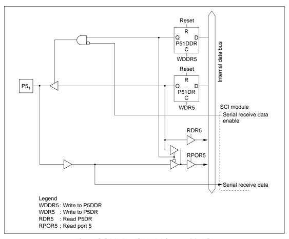
$Figure \ C-5 \ (b) \quad Port \ 5 \ Block \ Diagram \ (Pin \ P5_1)$
