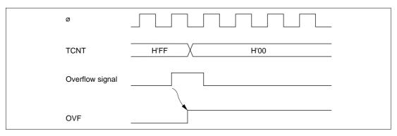
Figure 10-8 Timing of OVF Setting
