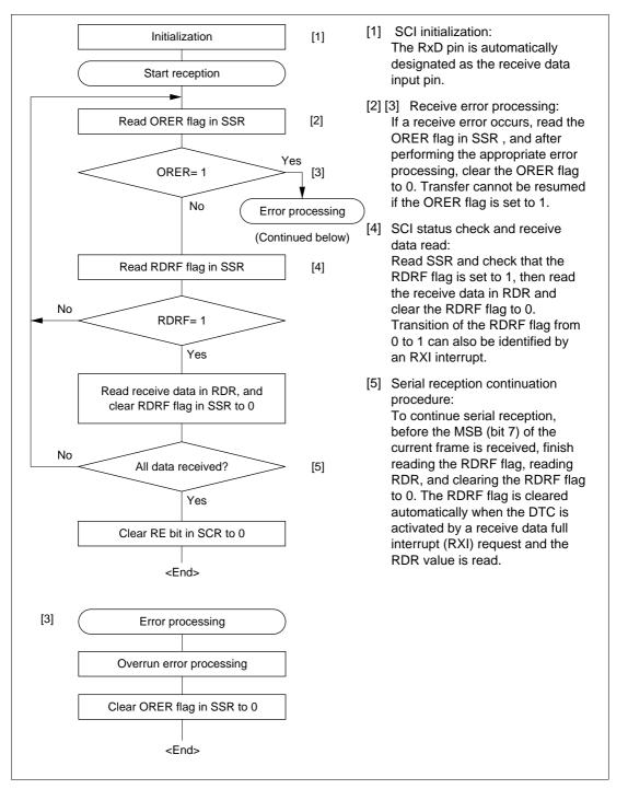
Figure 12-18 Sample Serial Reception Flowchart
