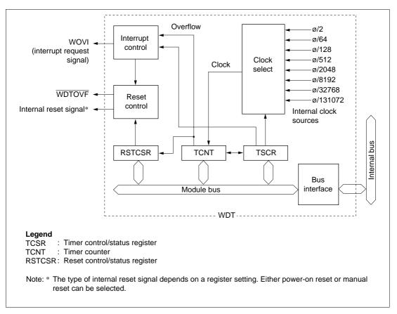
Figure 11-1 Block Diagram of WDT
