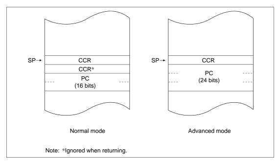
Figure 2-16 Stack Structure after Exception Handling (Examples)
