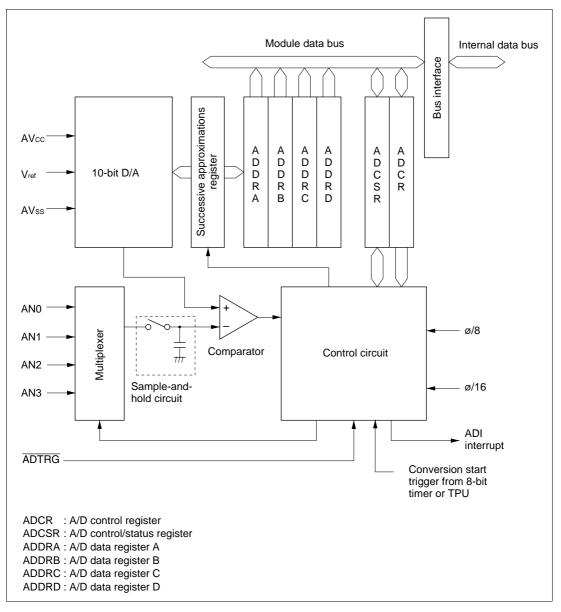
Figure 14-1 Block Diagram of A/D Converter
