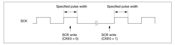
Figure 13-8 Timing for Fixing Clock Output Level
