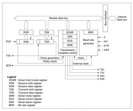
Figure 12-1 Block Diagram of SCI
