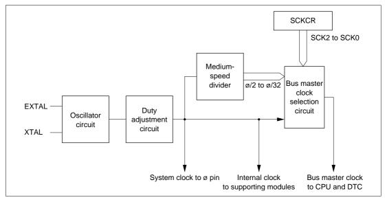
Figure 17-1 Block Diagram of Clock Pulse Generator
