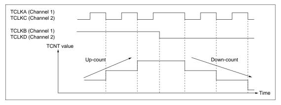
Figure 9-27 Example of Phase Counting Mode 2 Operation
