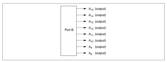
Figure 8-11 Port B Pin Functions (Modes 1, 4, and 5)
