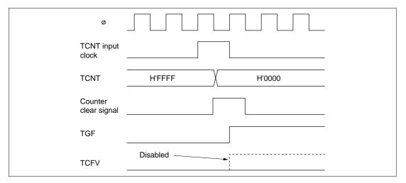
Figure 9-52 Contention between Overflow and Counter Clearing
