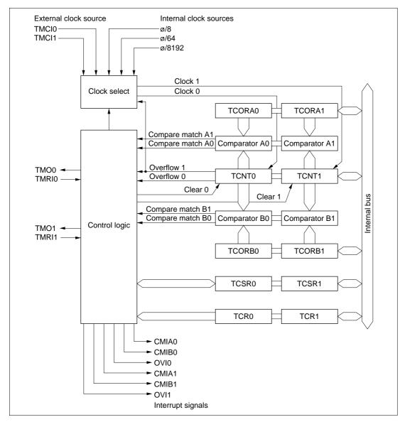
Figure 10-1 Block Diagram of 8-Bit Timer
