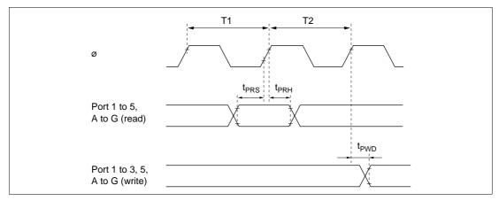
Figure 19-15 I/O Port Input/Output Timing
