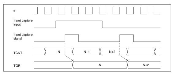
Figure 9-33 Input Capture Input Signal Timing
