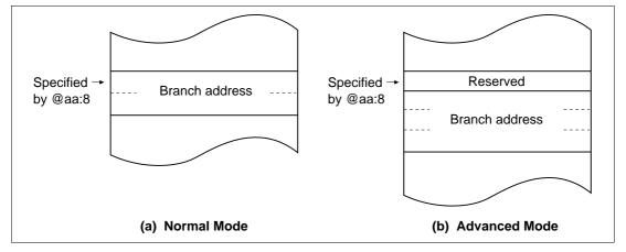
Figure 2-13 Branch Address Specification in Memory Indirect Mode
