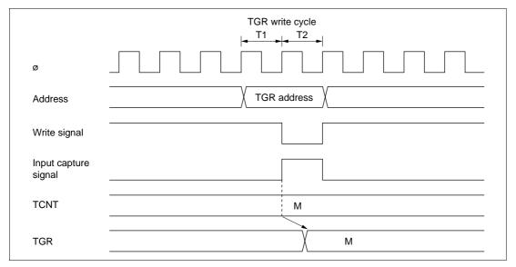
Figure 9-50 Contention between TGR Write and Input Capture
