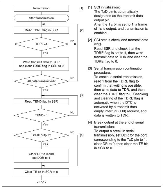
Figure 12-5 Sample Serial Transmission Flowchart
