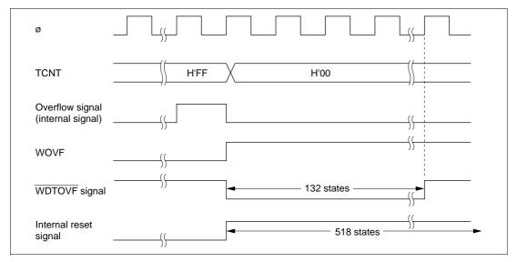
Figure 11-7 Timing of Setting of WOVF
