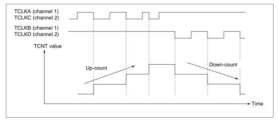
Figure 9-28 Example of Phase Counting Mode 3 Operation
