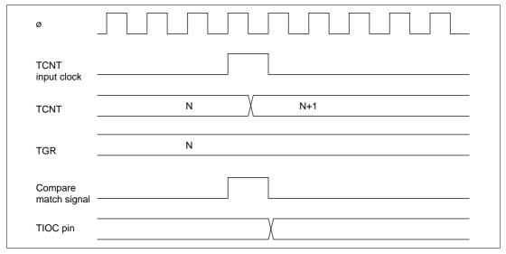
Figure 9-32 Output Compare Output Timing
