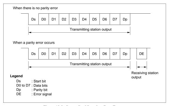
Figure 13-3 Smart Card Interface Data Format
