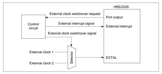
Figure 17-7 Sample External Clock Switching Circuit
