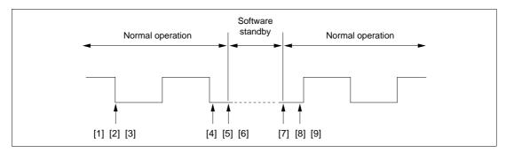
Figure 13-9 Clock Halt and Restart Procedure
