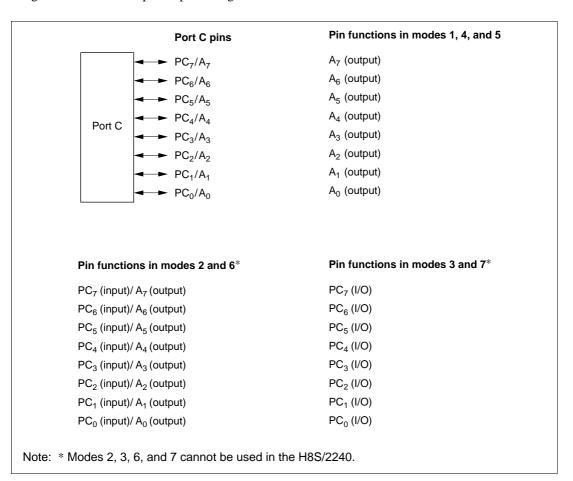
Figure 8-14 Port C Pin Functions
