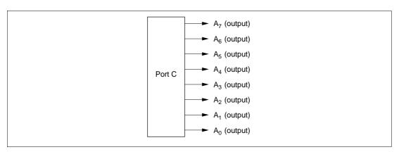
Figure 8-15 Port C Pin Functions (Modes 1, 4, and 5)
