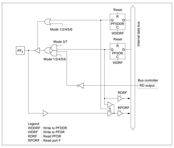
Figure C-11 (f) Port F Block Diagram (Pin PF<sub>5</sub>)
