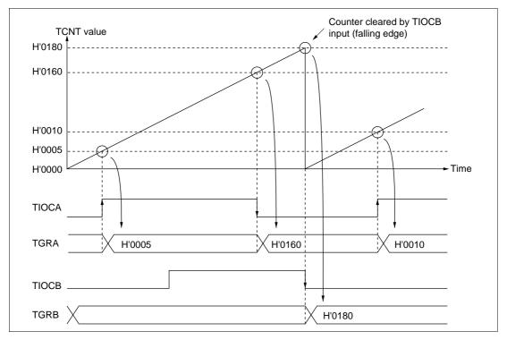
Figure 9-13 Example of Input Capture Operation
