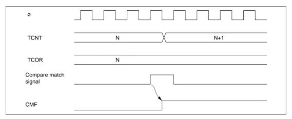
Figure 10-4 Timing of CMF Setting
