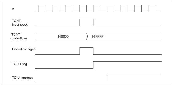
Figure 9-41 TCIU Interrupt Setting Timing
