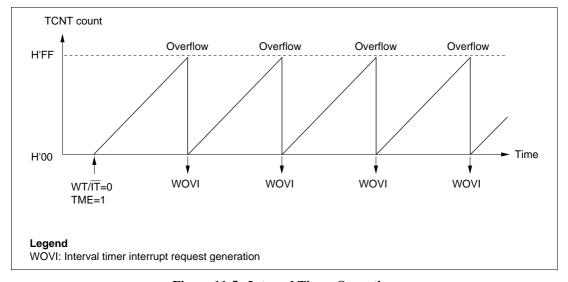
**Figure 11-5 Interval Timer Operation**
