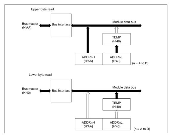
Figure 14-2 ADDR Access Operation (Reading H'AA40)
