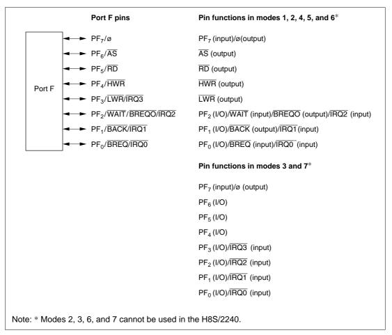
**Figure 8-24 Port F Pin Functions**
