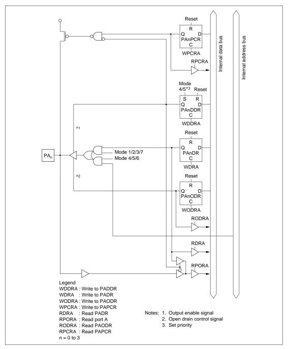
Figure C-6 Port A Block Diagram (Pins PA<sub>0</sub> to PA<sub>3</sub>)
