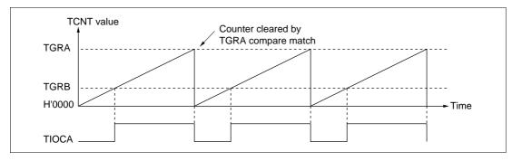
Figure 9-22 Example of PWM Mode Operation (1)
