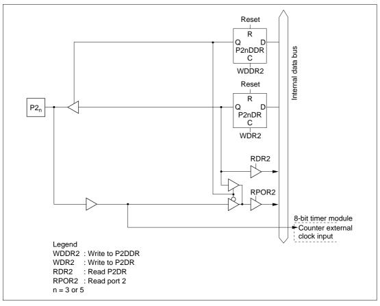
Figure C-2 (c) Port 2 Block Diagram (Pins P2<sub>3</sub> and P2<sub>5</sub>)
