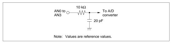
Figure 14-8 Analog Input Pin Equivalent Circuit
