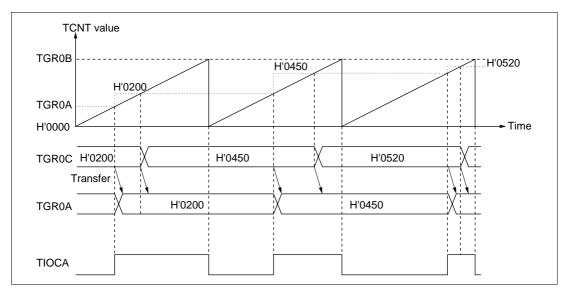
Figure 9-19 Example of Buffer Operation (1)
