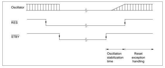
Figure 18-3 Hardware Standby Mode Timing (Example)
