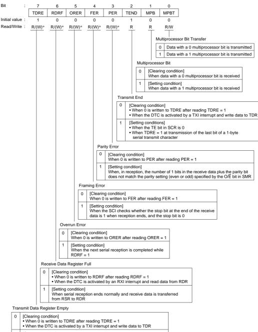
[Setting condition] . When the TE bit in SCR is 0 . When data is transferred from TDR to TSR and data can be written to TDR
