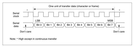
Figure 12-14 Data Format in Synchronous Communication
