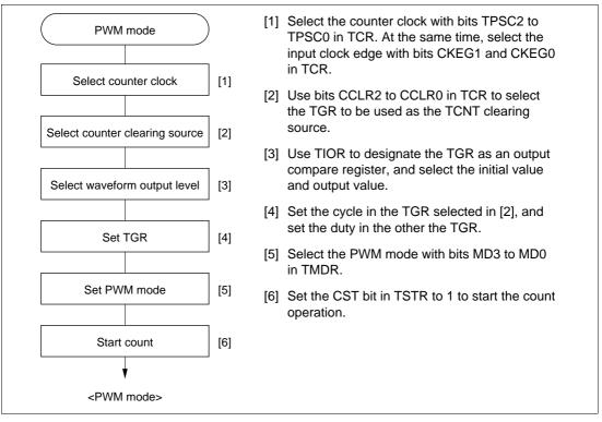
Figure 9-21 Example of PWM Mode Setting Procedure
