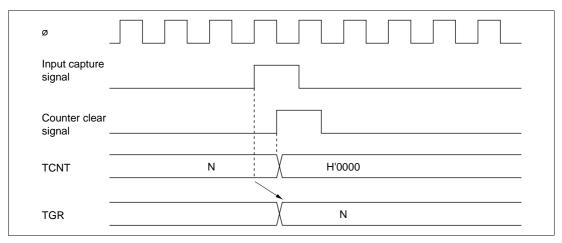
Figure 9-35 Counter Clear Timing (Input Capture)
