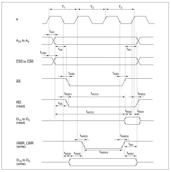
Figure 19-9 Basic Bus Timing (Three-State Access)
