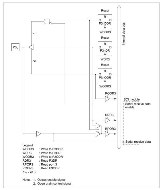
Figure C-3 (b) Port 3 Block Diagram (Pins P3<sub>2</sub> and P3<sub>3</sub>)
