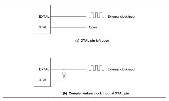
Figure 17-5 External Clock Input (Examples)
