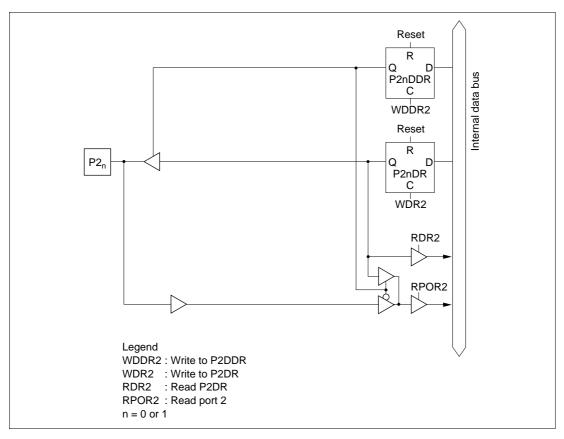
Figure C-2 (a) Port 2 Block Diagram (Pins P2<sub>0</sub> and P2<sub>1</sub>)
