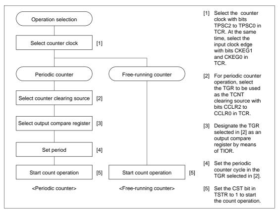
Figure 9-6 Example of Counter Operation Setting Procedure
