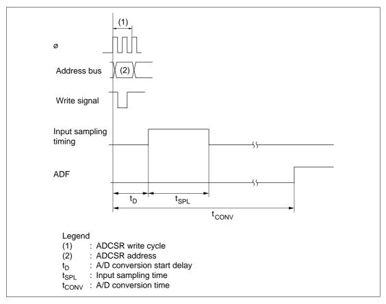
Figure 14-5 A/D Conversion Timing
