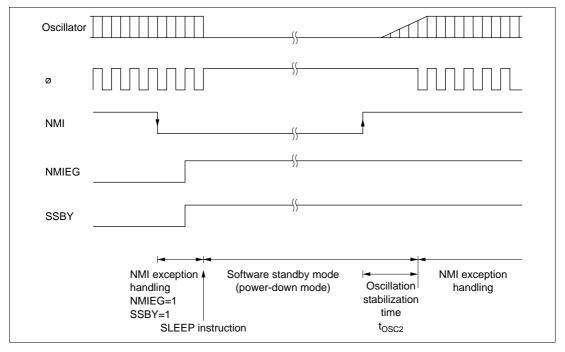
Figure 18-2 Software Standby Mode Application Example
